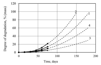
**Figure 3.** Estimated results of the degree of polystyrene biodegradation for a period of up to 6 months under the conditions of planned experiments
